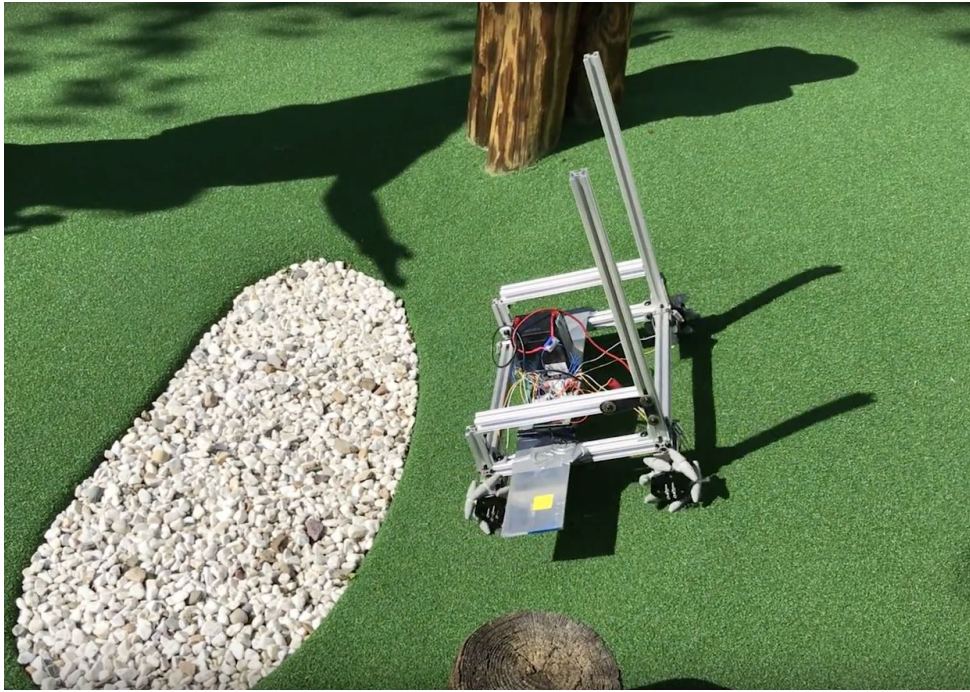
Figure 21 - Mecanum wheel testing apparatus
